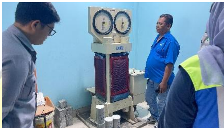
Gambar 3. 21 Uji Kuat Tekan Beton Reinforced Concrete Pipe (RCP) Sumber: Penulis (2026)
